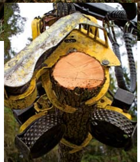
Feed rollers mainly carry the stem.
