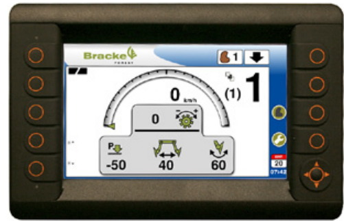
The operator can make settings and keep track of the trencher's functions with the display.
