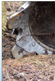
Discs with replaceable teeth.
