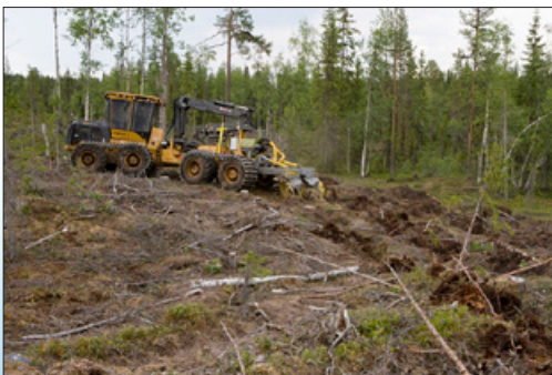
The Bracke T28.a is mounted on a medium-sized or large prime mover.
