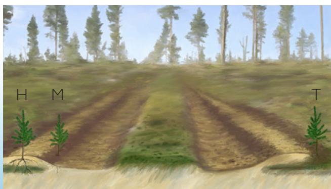
The Bracke T35.b creates planting spots with inverted humus (T), mineral soil mounds on inverted humus (H), and mineral soil mounds (M).
