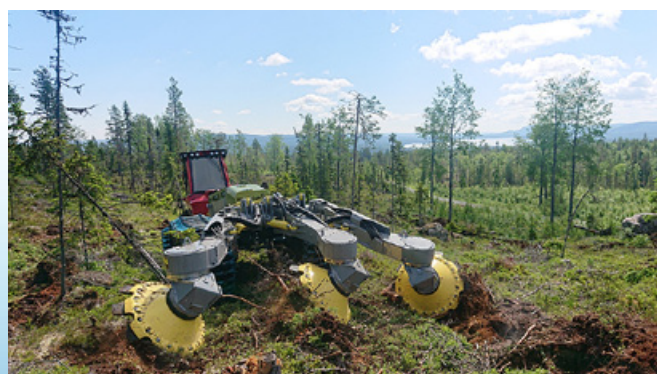
The Bracke T35.b is suitable for large scarification objects and is mounted on large prime movers.
