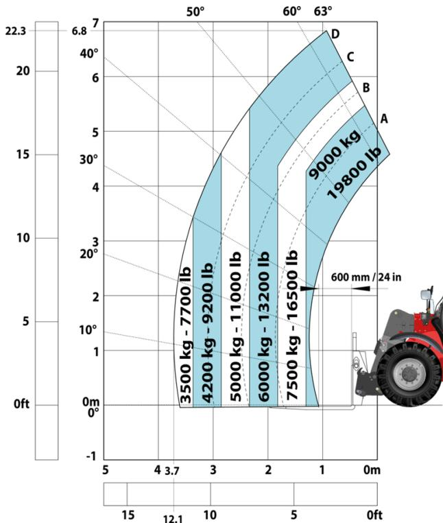
Machine on tyres with 3-hook jib 9000 kg (Metric)
