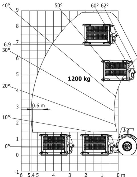
Machine on tyres with winch 9000 kg (Metric)
