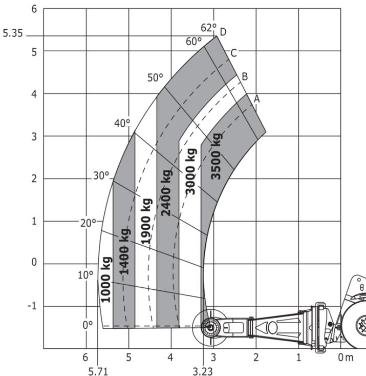
Machine on tyres with cylinder handler CH 4 (Metric)
