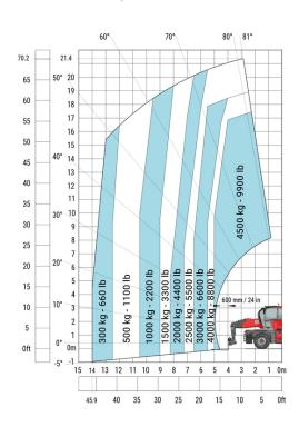
Machine on lowered stabilisers with 1500 kg jib with winch (Metric)
