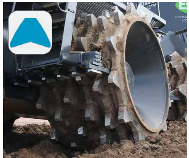
BOMAG wheels with weld on teeth.
