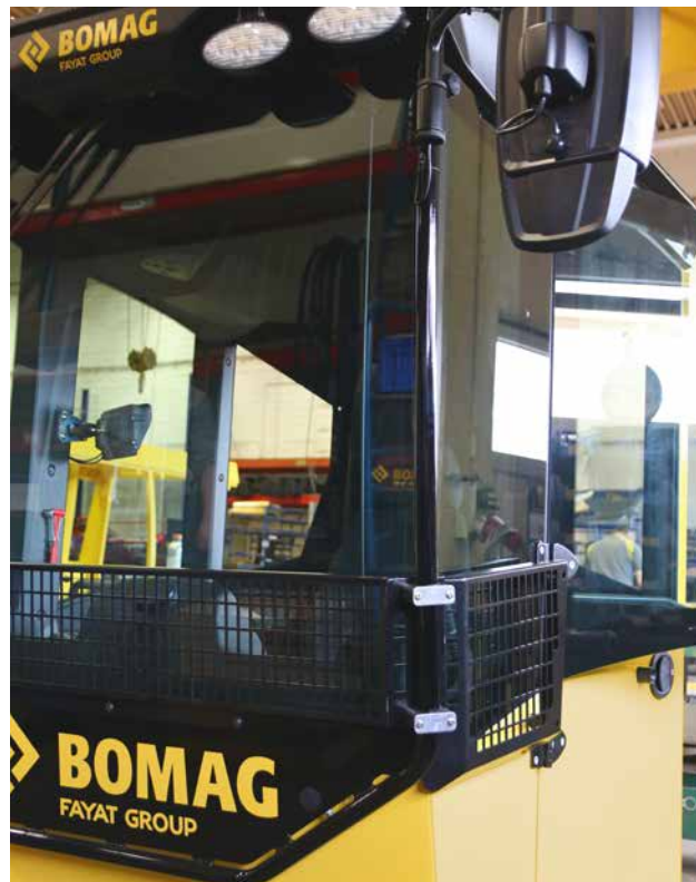
Cab protection grille protects damage to the cab windows.
