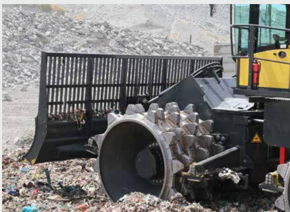
Scrapers ensure clean wheels and high compaction.
