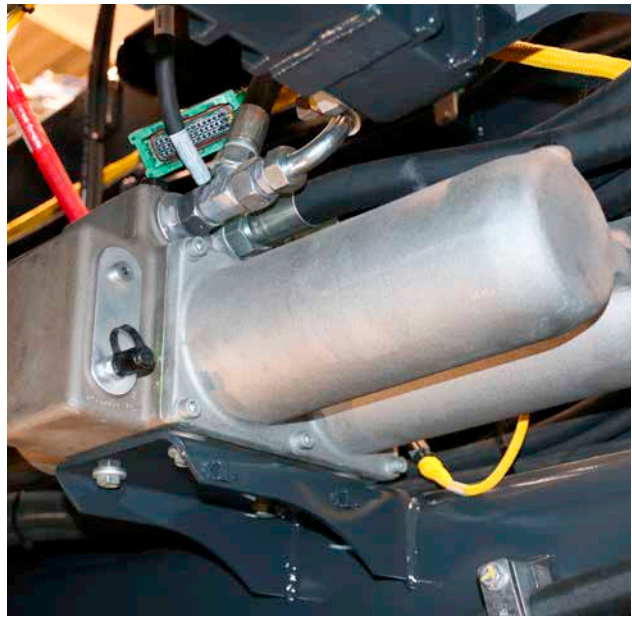
Electronic monitoring of hydraulic return filter.
