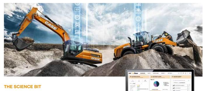
The CASE SiteWatch telematics system uses a high-tech control unit mounted on each machine to collate information from that machine and from GPS satellites. This data is then sent wirelessly through the mobile communication networks to the CASE Telematics Web Portal.
