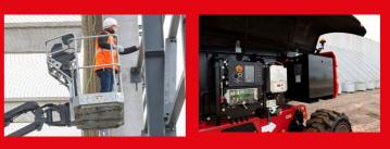
Basket 1.8 m with lateral door Manitou offers a wider basket with a side door for easy access.
