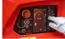
The large screen at the lower control box offers additional information to the top control box for operator and allows technicians to carry out a quick diagnosis, consult the machine memory and many other functions.
