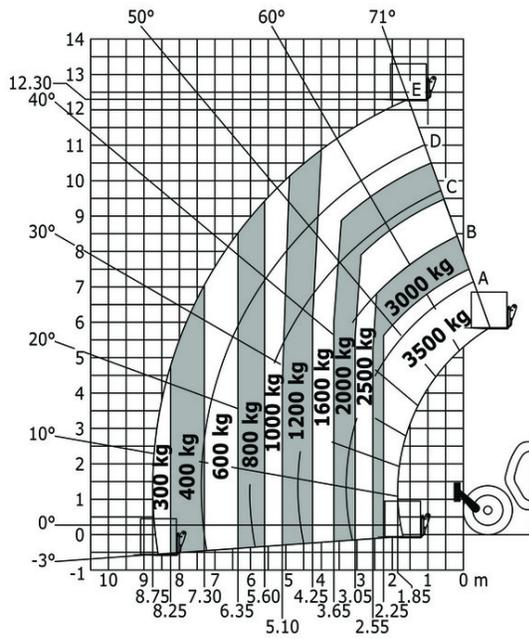
Machine on stabilizers with forks Metric
