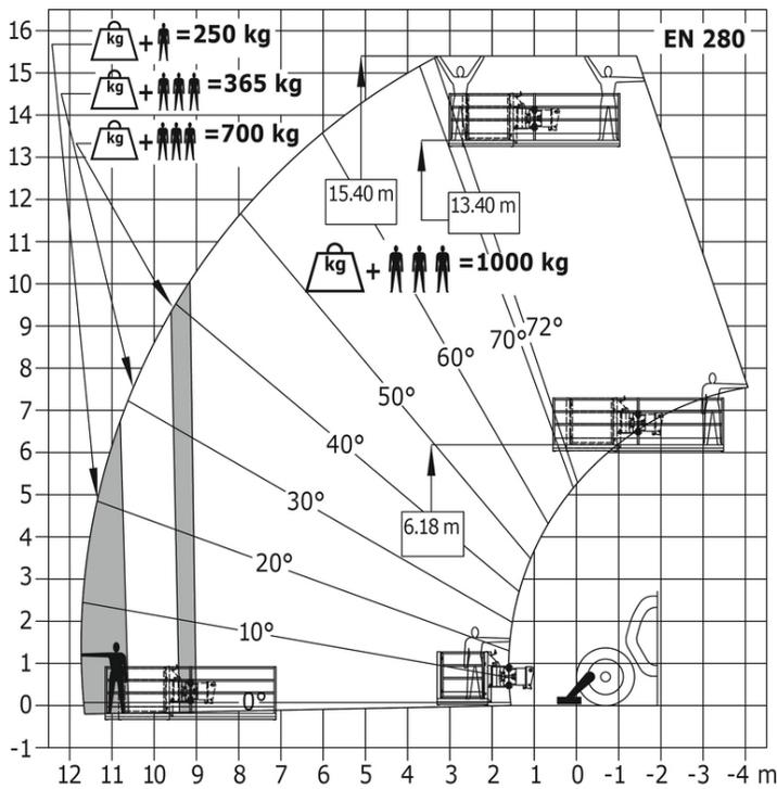
Machine on tyres with forks - with levelling Metric
