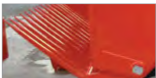
■ Lateral shear + double tines on sides for easy cutting operations
