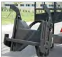
■ Hydraulic rib clamp-opening 325 - 482mm
