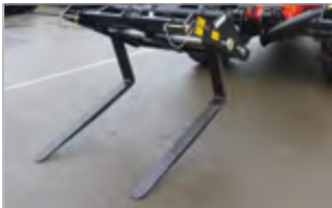
■ Floating forks with levelling
